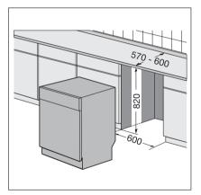
By removing the machine's worktop, you can install it under a close fitting sink unit or a pre-existing top, providing the dimensions of the recess correspond to those shown in the picture.
